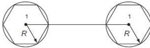
Fig.4.14 | Frequency reuse ratio q = D/R
